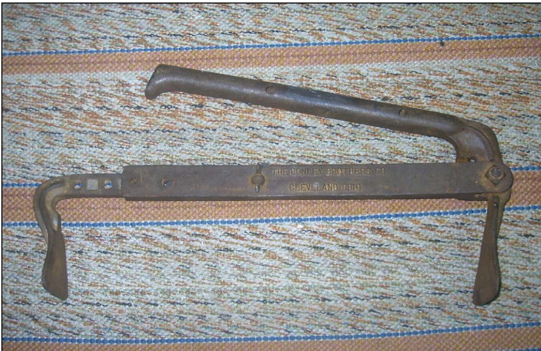
Antique brick mason tool for carrying a load of bricks
