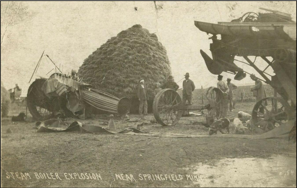
Farming is a dangerous occupation. Here is an old postcard that shows the remnants of a steam boiler explosion near Springfield, Minnesota.
